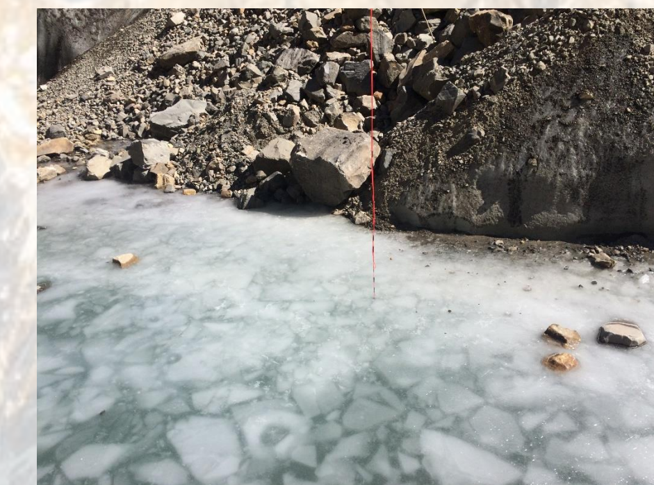
Figure 2. Tiny tag temperature sensors were installed in 7 supraglacial ponds. This gave an hourly temperature record for the 3 week field season
