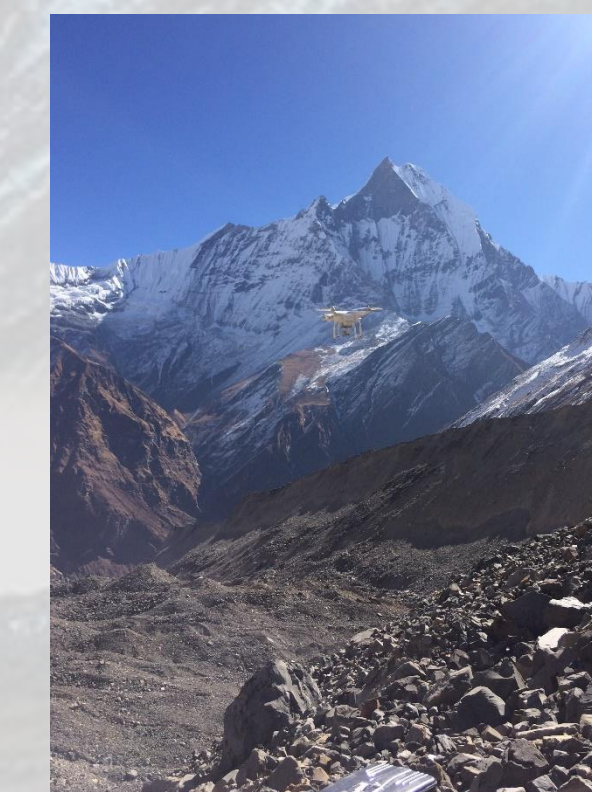
Figure 4. Drone survey of the glacier surface of Annapurna South Glacier. This produced a 3D model of the whole glacier surface with ~3cm accuracy
